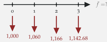
Figure 4.1. The price paid per tonne of reagent in each of the four years. The average inflation rate is the single growth rate that connects the first arrow to the last.
